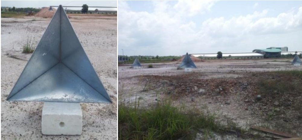
Figure 6. Test Site with Four Trihedral Corner Reflectors as Radar Targets
