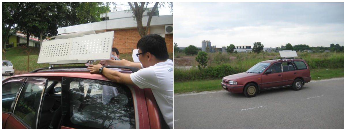
Figure 5. Ground-based Truck-Mounted SAR Imaging Experiment
