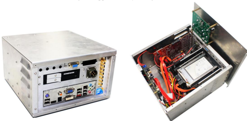
Figure 3. Hardware Prototype of the Embedded SAR Processing Module
