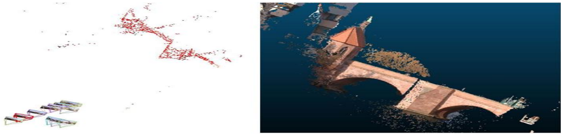
Figure 3. 3D reconstruction via VisualSFM (left); Close-range photogrammetry point clouds (right)
