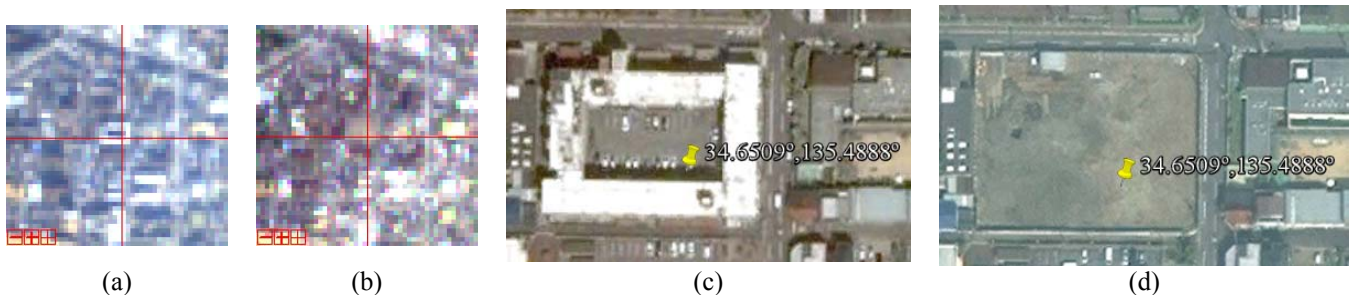
Figure 6. An example of negative change detection for Osaka dataset. (a, b) 4 \times magnified AVNIR-2 true color composite image acquired on 2/12/2008 and 18/5/2009, respectively. (c, d) QuickBird image from Google Earth. Red crosshair and yellow pin denote the negative change which backscatter decreased.
