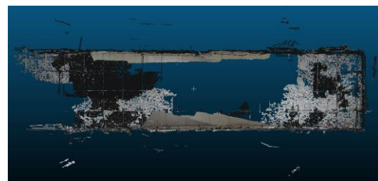
Figure 10: Combined point cloud after adjusted manually
