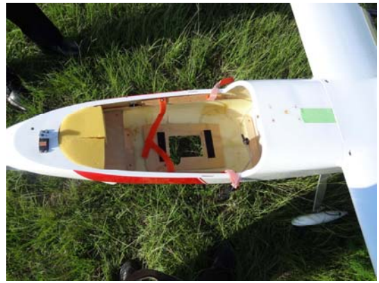
Fig. 5 Front side photo of the unmanned airplane and observing hole
