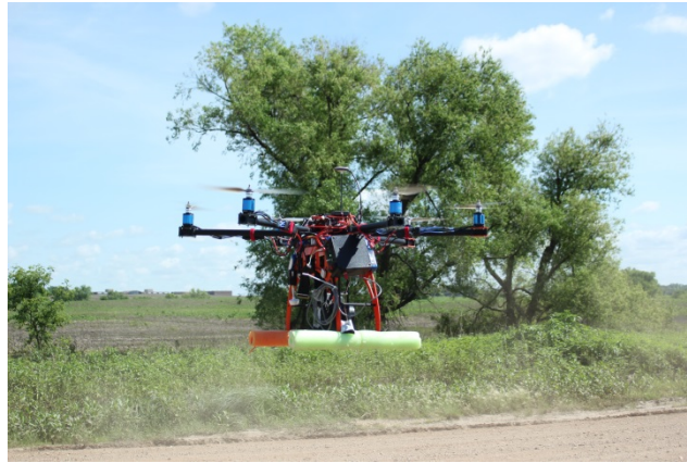
Figure 2: The selected Bergen hexacopter UAV being used to measure unpaved road condition in South Dakota, USA.
