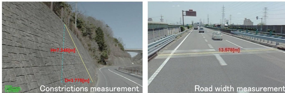
Fig. 6 Measurement by high-resolution 360 degree full spherical geo-referenced video
