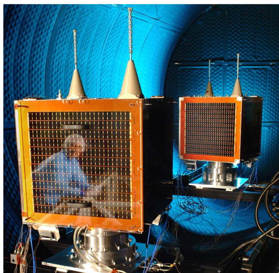
Fig.7 1st generation DMC satellites under test
