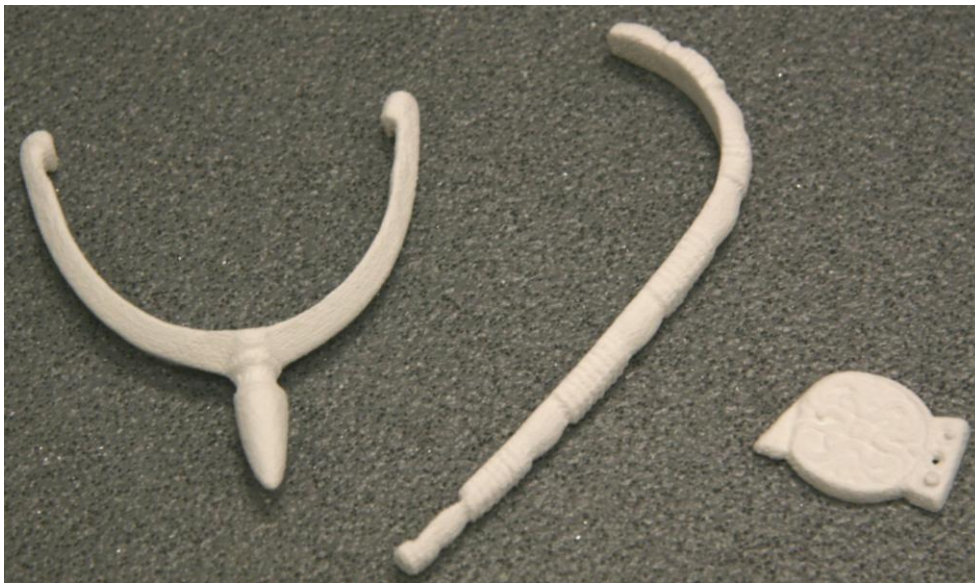
Fig.3 Models of bronze artifacts created on Zprinter 450
