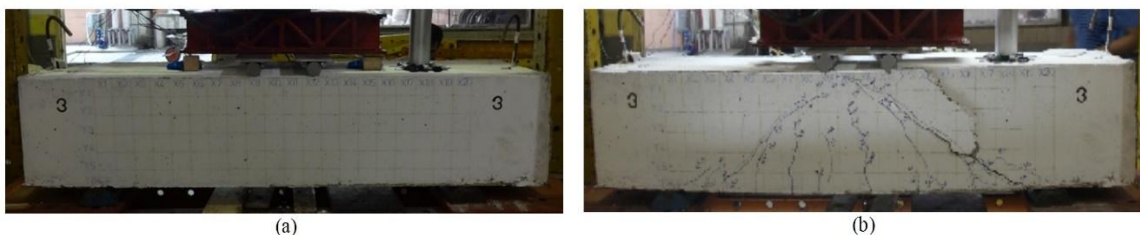
Figure 3. Reinforced concrete beam (a) Pre-stressed, (b) Failure
