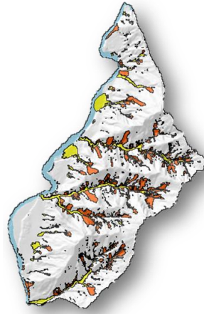
Figure 3. Landslide inventory mapped manually with separating landslides (in orange) and runouts (in yellow).
