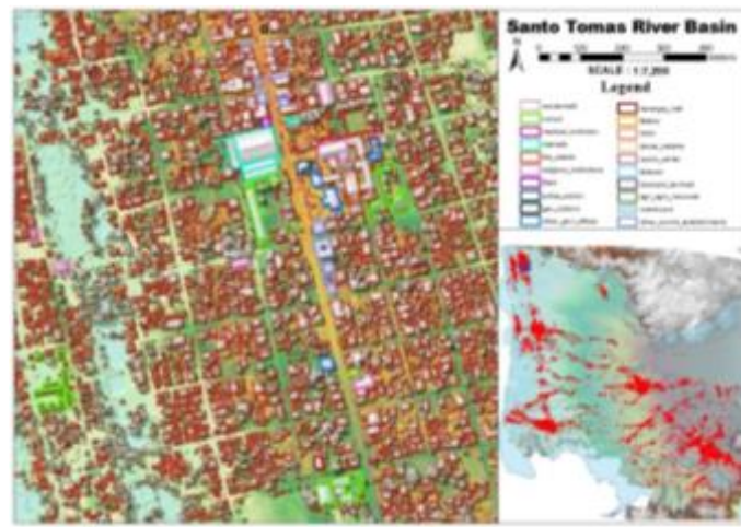
Figure 3. The extracted building footprints in the flood plains of Santo Tomas River.
