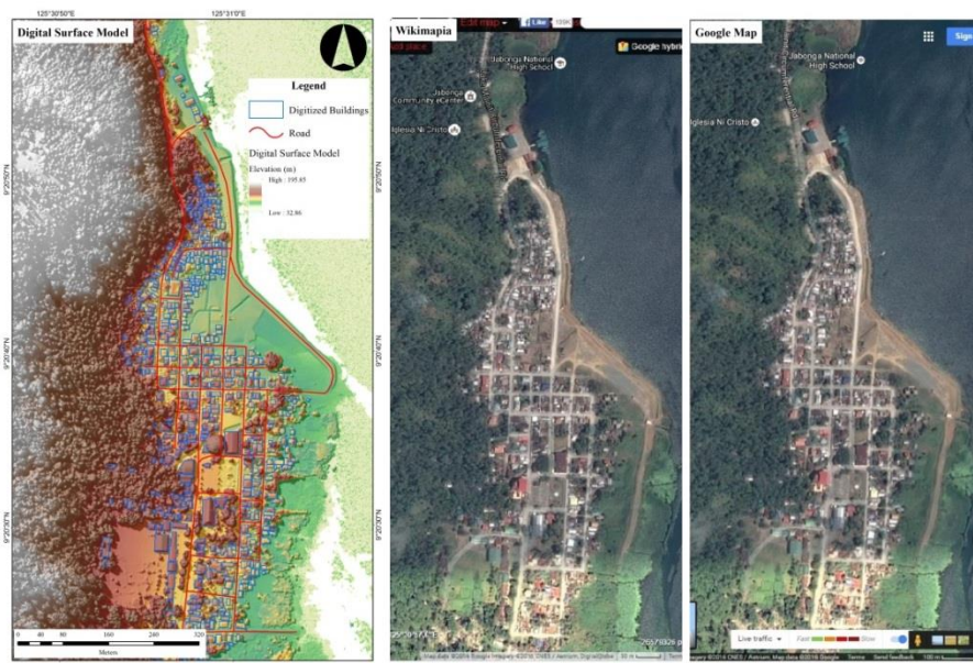
Figure 2. The LiDAR DSM of a portion of Jabonga Municipality (left), Wikimapia screenshot (middle) and Google Map screenshot (right) that were used in building attribution.
