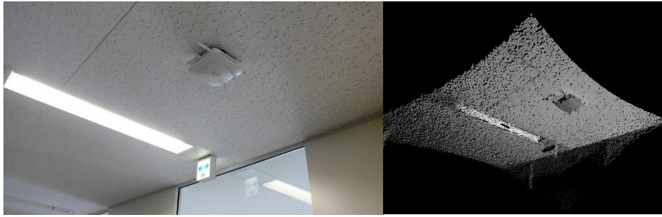
Figure 9. Wi-Fi router (left image: photo, right image: point cloud)
