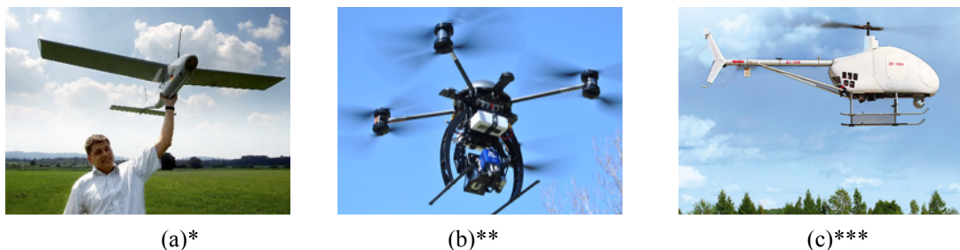
Figure 2. Types of UAV used in remote sensing: a) fixed wing b) multi-rotor c) single-rotor
