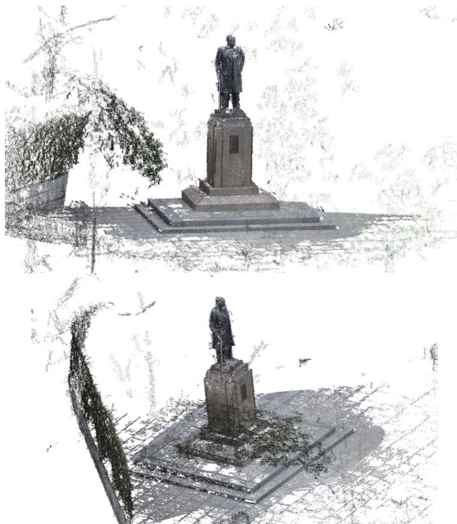
Figure 14. Generated point cloud of a bronze statue
