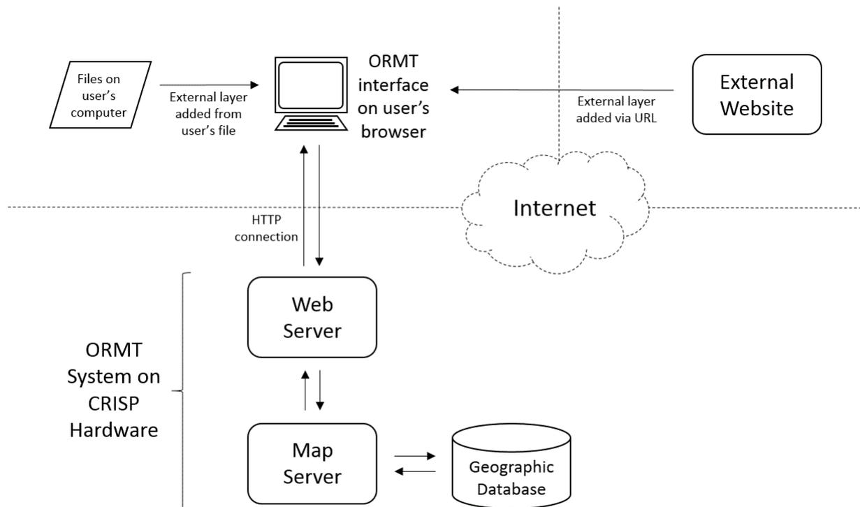
Figure 1. Outline of the ORMT system. When the user accesses the ORMT via web browser, the user interface is loaded onto the browser. Users may add external layers by specifying a URL, or by selecting a file on their computer. Datasets provided by the ORMT are stored in the geographic database and served by the map server to the user's browser via HTTP.
