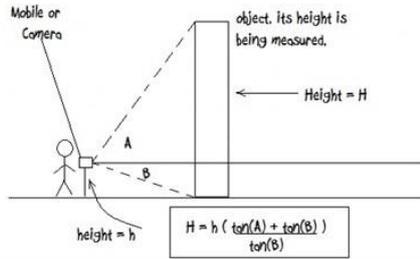
Fig. 1. KDD's solution in getting the height of an object
