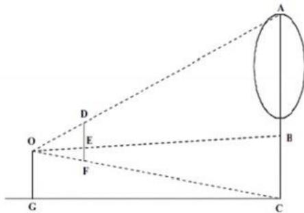
Fig.2 Geometric method principle in computing height
