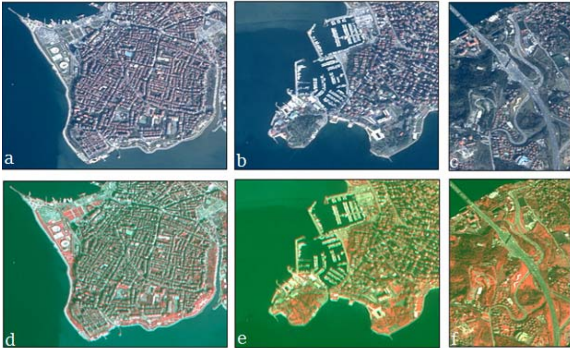
Figure 1. The subset of the test area (R: red band, G: Green band, B: Blue band) (a, b, c) and (R: NIR band, G: Green band, B: Blue band) (d, e, f)
