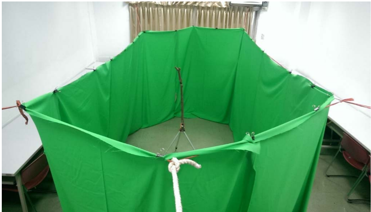
Figure 1 Experimental set-up of the “green” room (for taking pictures of roots)
