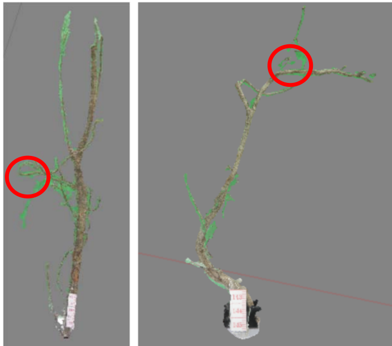
Figure 10 Incomplete shape and missing branches of root model due to the shadowing effect of other branches (view obscured by other branches in original photos)
