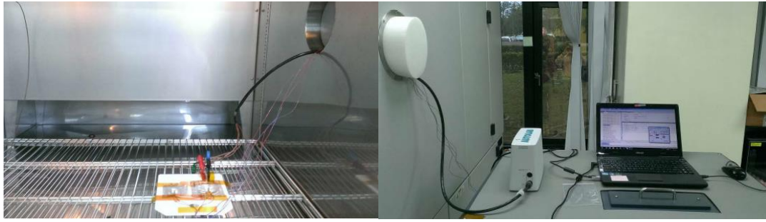
Fig. 7 Soft pack lithium-sulfur battery and battery charge/discharge device
