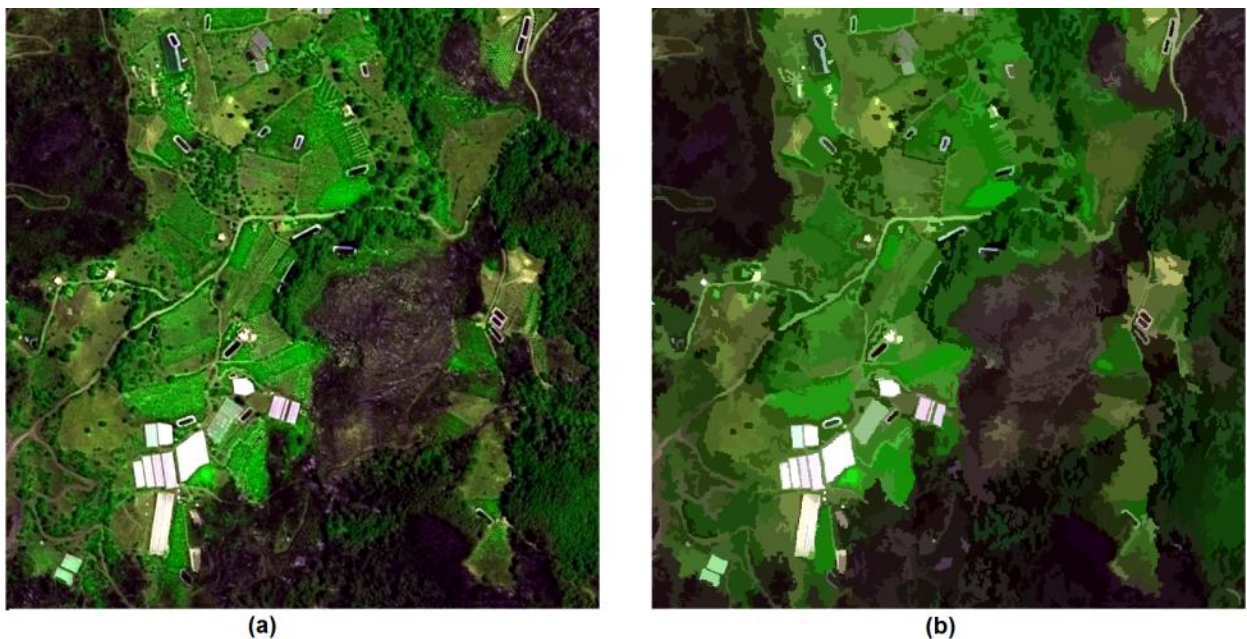
Figure 3. Spot 6 image before – after segmentation process; a) pixel view, b) segment view.
