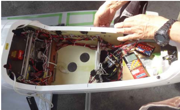
Fig. 10 Observation holes at the aircraft body
