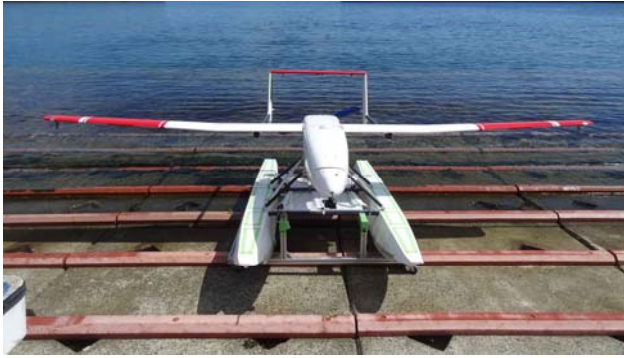
Fig. 8 Aircraft type UAV with 2 floats for the taking off and landing at water (Front)
