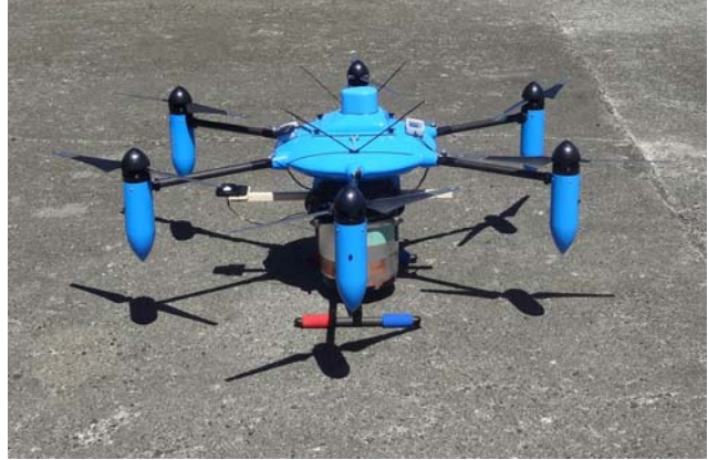
Fig. 14 The hyperspectral sensor with multi-copter
