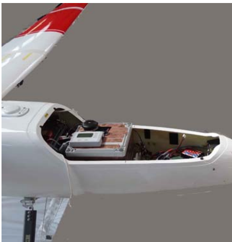
Fig. 11 The sensor set in the aircraft body (Side)
