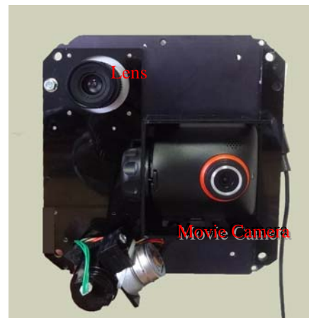
Fig. 5 Bottom side photo of the hyperspectral image sensor
