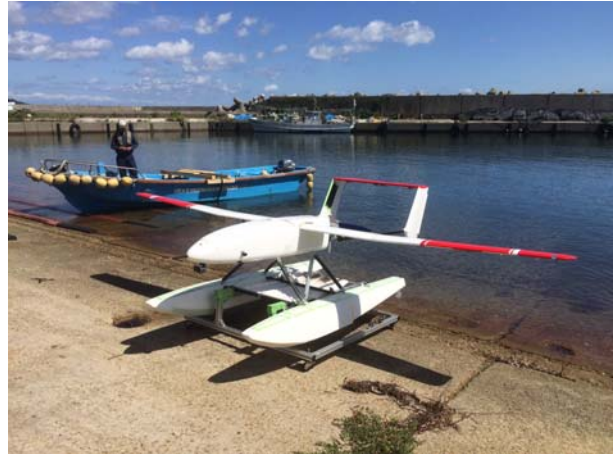
Fig. 9 Aircraft type UAV with 2 floats for the taking off and landing at water (Side)
