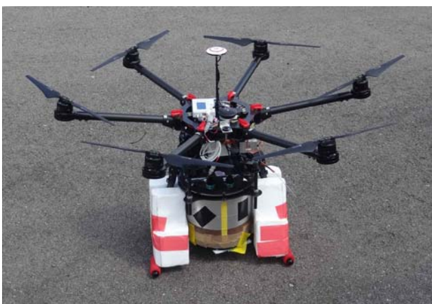
Fig. 17 The sensor was mounted with ordinary multi-copter
