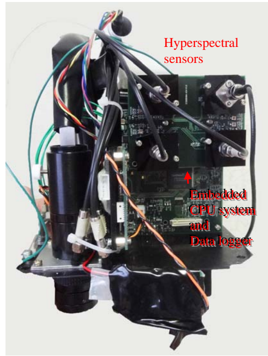
Fig. 3 Left side photo of the hyperspectral image sensor
