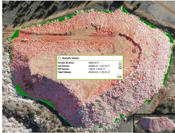
Figure 7: Volumetric calculation for stockpile
