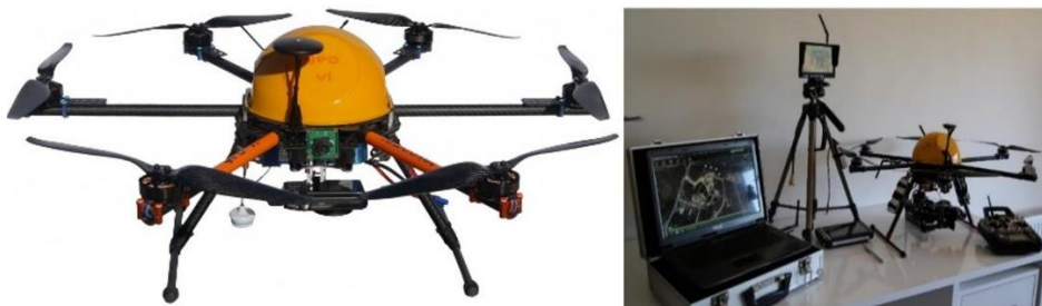
Figure 2: Hexacopter UAV and other equipments
