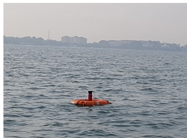
Figure 1. Aquadopp 2Mhz current meter deployment.
