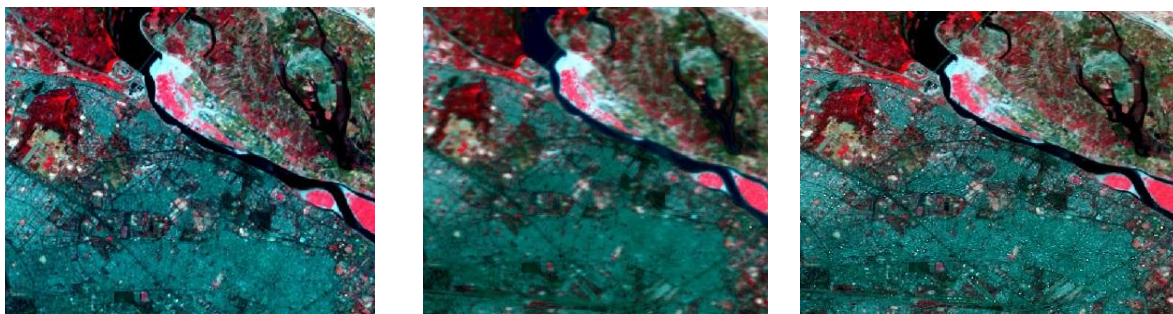
Figure 4: Subsets of (i) sentinel 2A (ii) Ehler and (iii) HPF fused image
