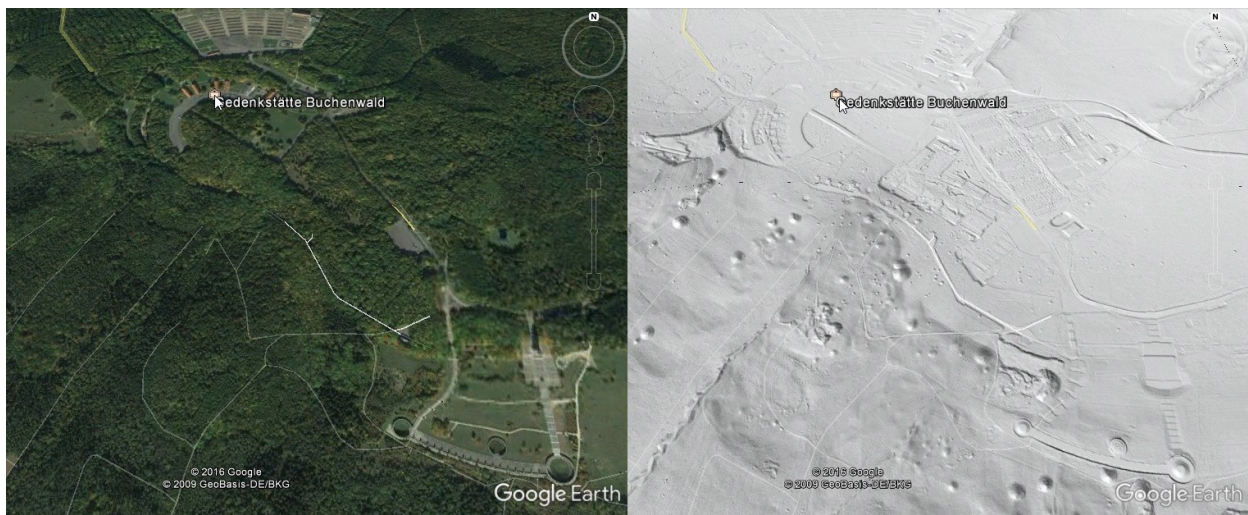
Figure 4: Comparing aerial imagery from Google Earth with the hillshaded DTMs generated from the LiDAR.
