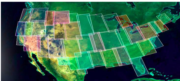
Figure 4. Simulation of complete coverage of CONUS in a fortnightly period with DEIMOS-1
