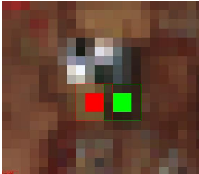
Figure 6 Two targets identified in L8-OLI image. “Pure pixels” are filled with solid color, “red” for red soil and “green” for black soil. Outline line shows the total pixels for each target type.
