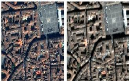
Fig. 7 Fused image using B-spline and super curve, fused image using weighted mean respectively.
