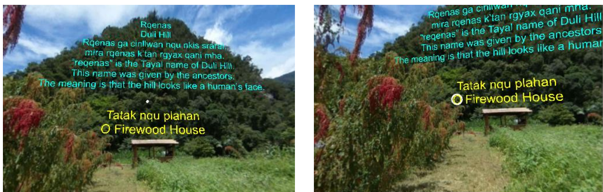
Figure 5. User interface (The white dot in the left figure is the center of user's sight. When user turns around to let the white dot aim at the yellow circle beside “Firewood House”, the white dot will turn into a small white circle.
