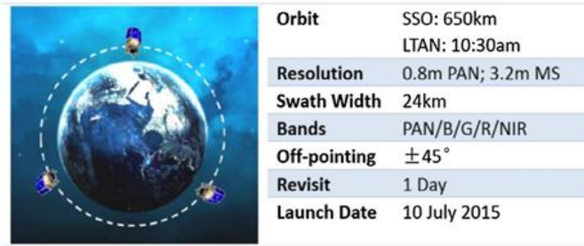
Figure 3. Diagram of Triplesat constellation orbit and specification.
