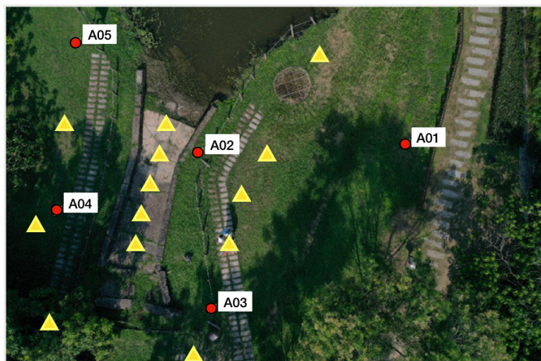
Figure 2. Location Of Each Scan Station (Yellow Triangle Icon) And GCPs (Red Circle Icon)
