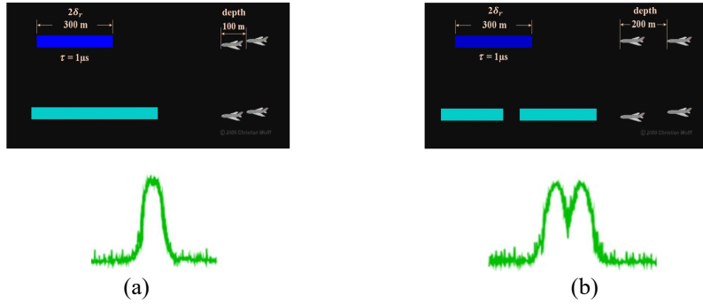
Figure 2. Illustrations of range resolution (revised from Wolff, 2009): (a) the depth is shorter than the range resolution and results in a deformed laser pulse return; (b) the depth is longer than the range resolution and a deformed pulse return with two wave crests is obtained.
