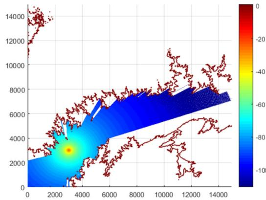
Figure 6 Calculated EM field of cut plane height of 100 m and area of 500 x 500 cells with the cell size = 30 meters. The base station located at cell x = 100 and y = 100.
