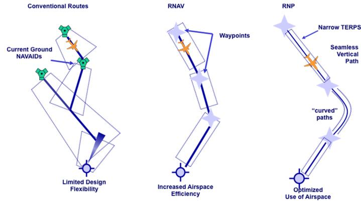
Figure 1 Conventional aircraft navigation and PBN navigation (RNAV and RNP)
