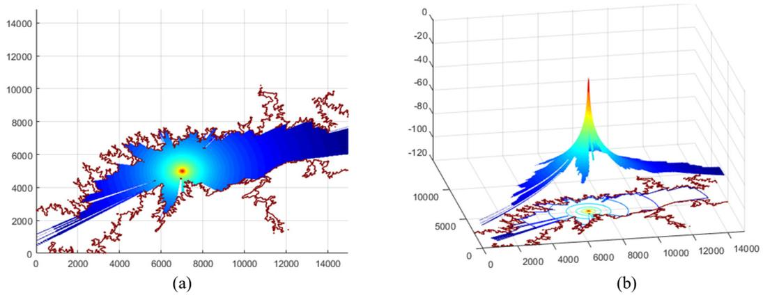
Figure 8 Calculated electric field of cut plane height of 85 m and area of 500x 500 cells with the cell size =30 meters. The base station located at cell  $x = 233$  and  $y = 166$  (a) top view (b) perspective view.
