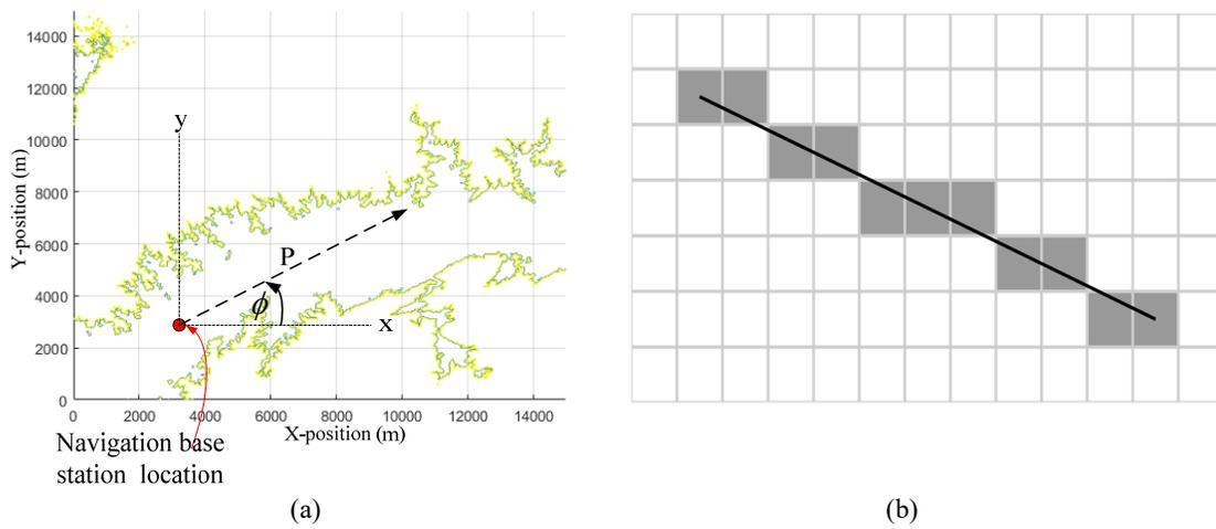
Figure 4 3D grid based line-of-sight search algorithm (Tx location and parameter) (b) Bresenham's line algorithm [2].
