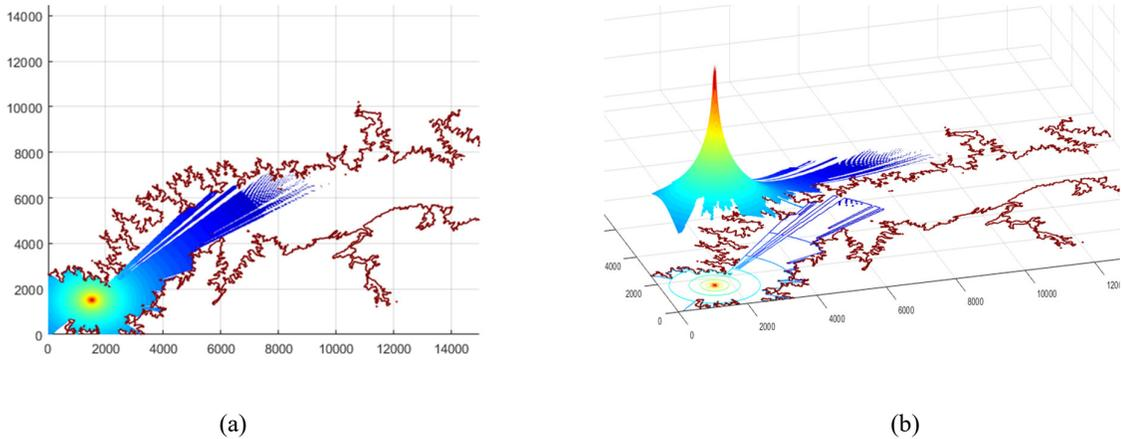
Figure 7 Calculated EM field of cut plane height of 85 m and area of 500 x 500 cells with the cell size = 30 meters. The base station located at cell x = 50 and y = 50 (a) top view (b) perspective view.
