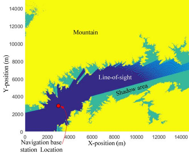
Figure 5 Results of the proposed searching subroutine of an airplane flight altitude of 100 meters.
