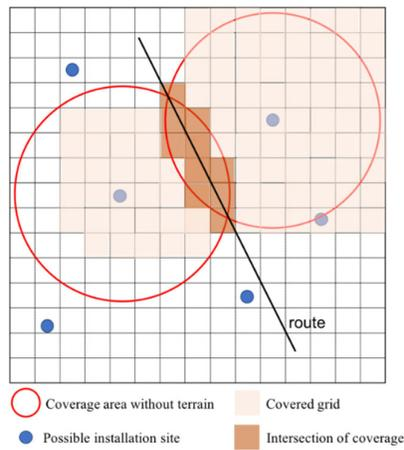
Figure 9 Example of grid airspace with candidate installation sites and signal coverage.
