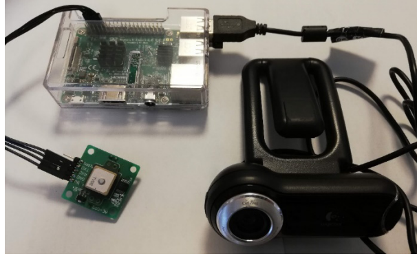
Fig. 1 Raspberry Pi, camera, and GPS module used for the prototype creation
