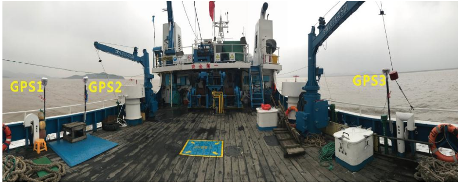
Figure 5 Tide measurement with Ship borne GPS receivers
