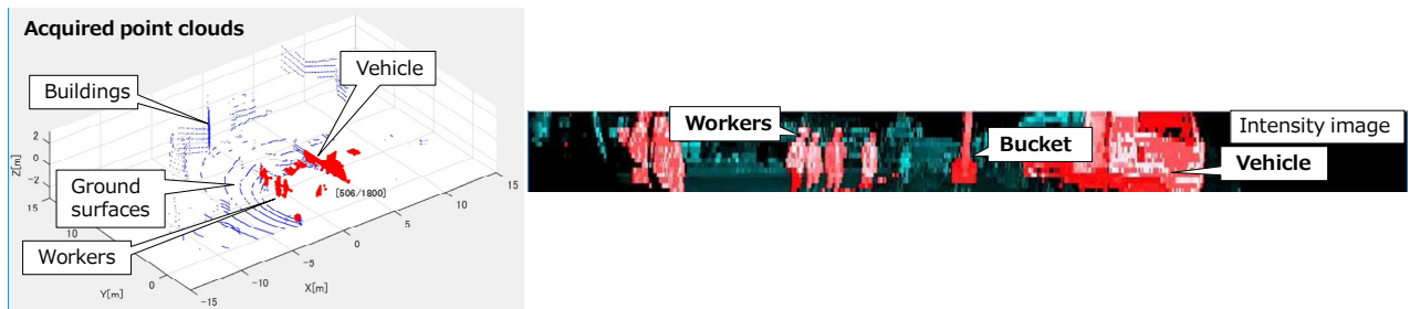
Figure 8. Acquired point clouds and extracted moving objects
