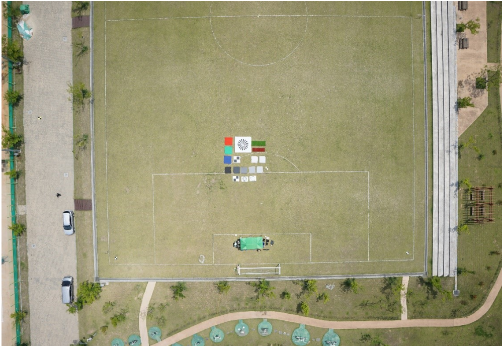
Figure 3. A multispectral image acquired using A5100 camera on a quad-copter at 100 m altitude.
