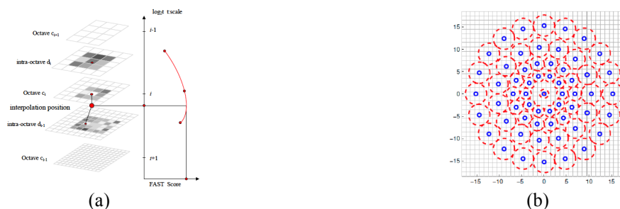
Figure 2. The generation of a BRISK features and its sampling pattern (Leutenegger et al., 2011)
