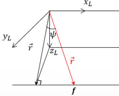
Figure 2 Doppler centroid and azimuth squint angle
