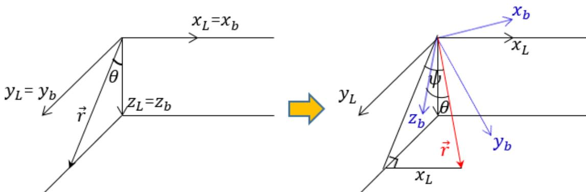
Figure 1 Variation of beam pointing geometry due to satellite attitude rotation
