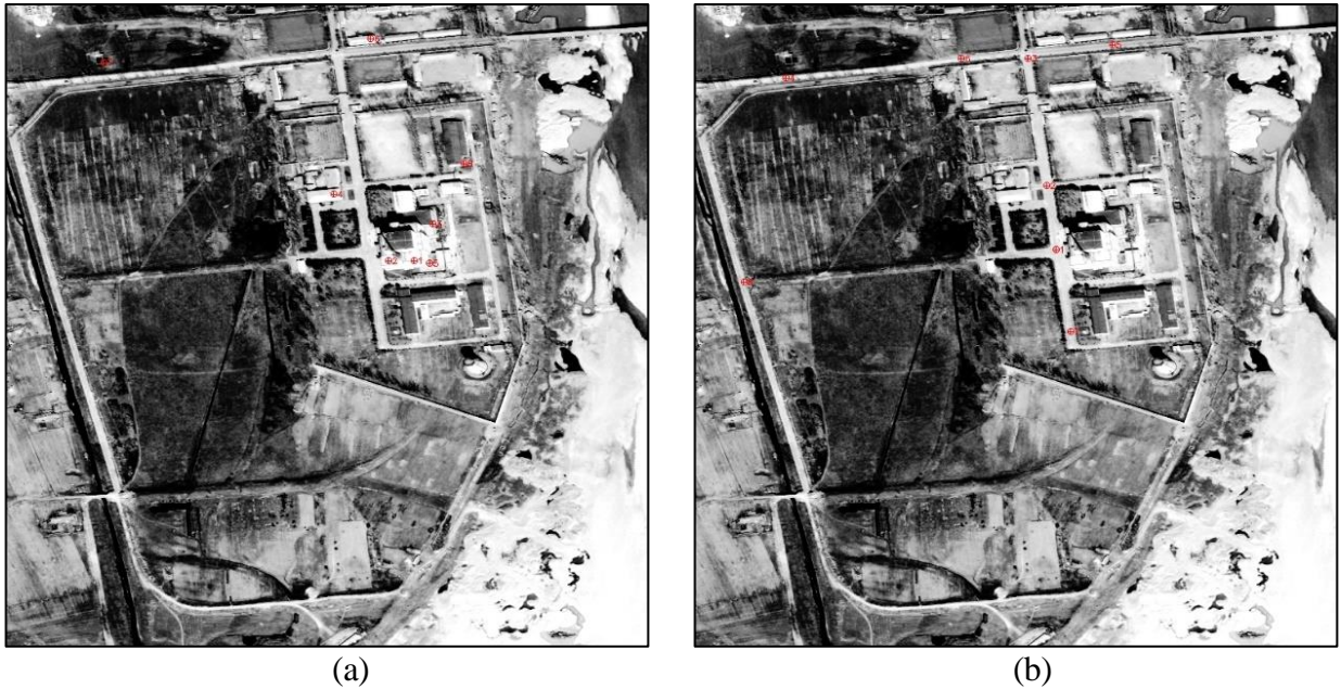
Figure 6: Reference images to evaluate RMSE showing the CPs with different criteria: (a) building oriented and (b) road network-oriented.
