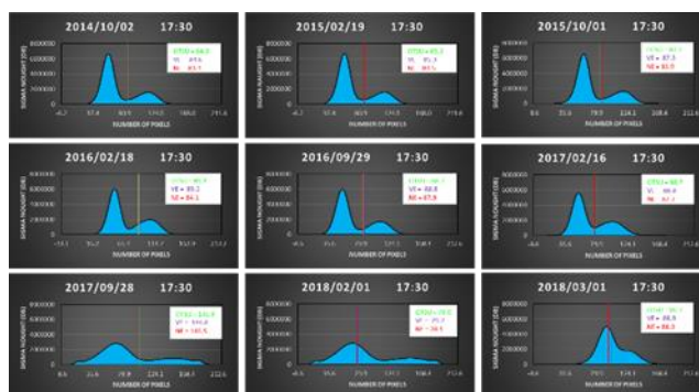
Figure 8 The weigh average of HH+HV applied on the whole area Green indicate OTSU threshold, Purple shows VE threshold and Red represent NE threshold
