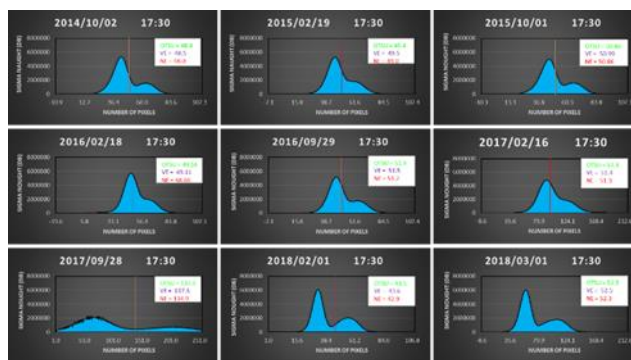
Figure 7 The weigh average of HH applied on the whole area Green indicate OTSU threshold, Purple shows VE threshold and Red represent NE threshold
