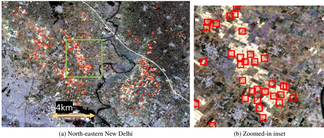
**Figure 6: Brick kilns around New Delhi identified by the current methodology. Brick kilns detected in the north-eastern portion of New Delhi (a) and a zoomed-in view (b) of the detection.**
