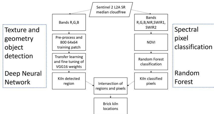
**Figure 2: Processing flowchart for identification of brick kiln.**
