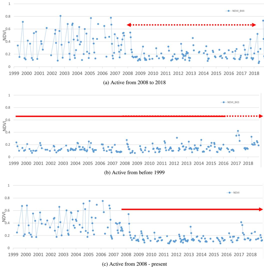
**Figure 8: NDVI calculated over the brick kiln locations reflect brick kiln’s age of operation as shown in (a) 2008-2018, (b) always active and (c) active since 2008. Solid line denote active period, dotted line denotes currently inactive brick kiln.**
