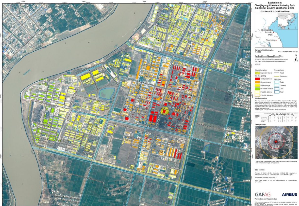
Figure 9: Damage assessment map of Chenjiagang Chemical Industry Park based on Périades-1B satellite acquired on 24/03/2019
