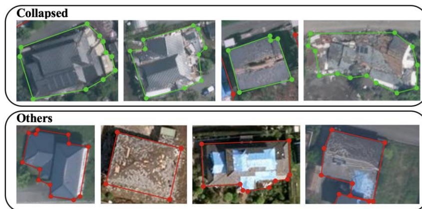
Figure 3 Examples of the buildings labeled in two different damage levels
