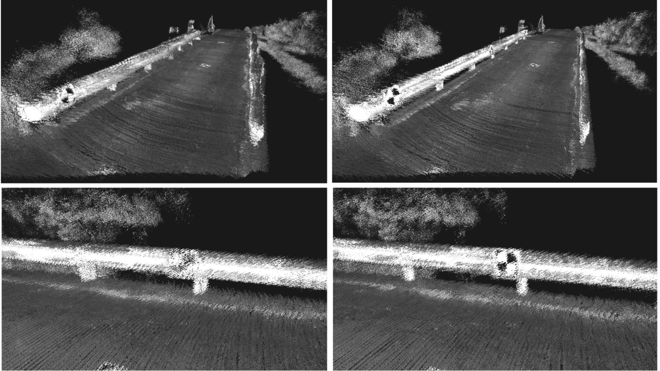
Figure 15. Registered point clouds (left: initial registration result, and right: fine registration result)
