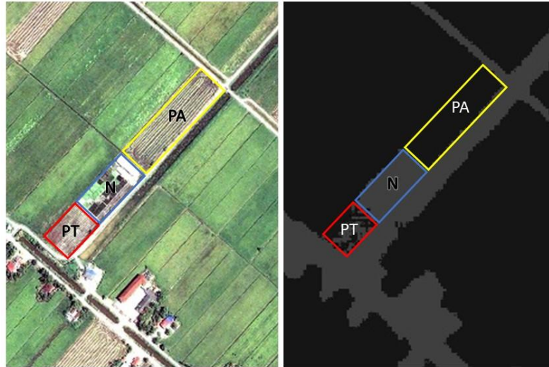
Figure 5: Output sample of the semantic segmentation networks on paddy fields. First column: Input image, second column: FCN output
