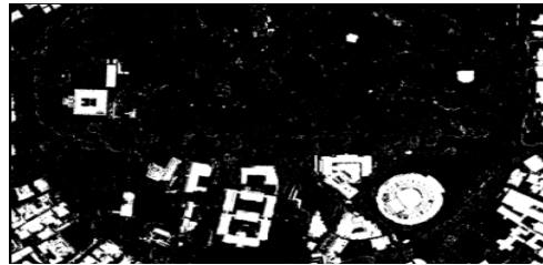
Figure 7 Automatic extracted building using transformation model from LIDAR point cloud and high resolution optical image
