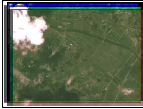
Figure 4. Misalignment of the green and red CCDs with respect to blue.
