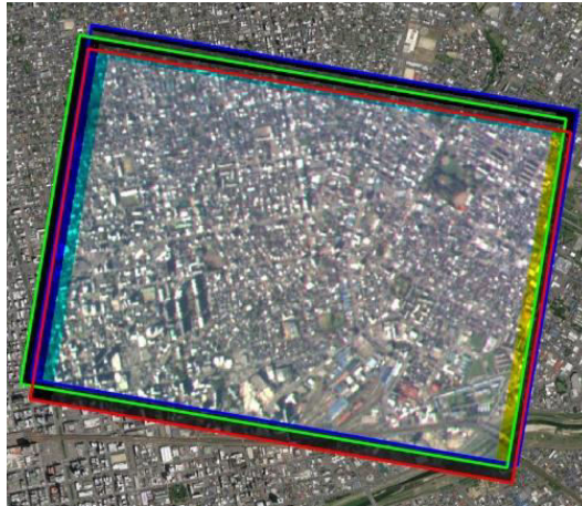
Figure 1. Georeferenced Diwata-2 HPT data showing the misalignment of bands.
